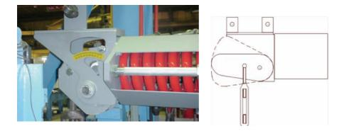
As the pipe moves further away from the fulcrum its weight must reduce if the seesaw is to remain in balance.
